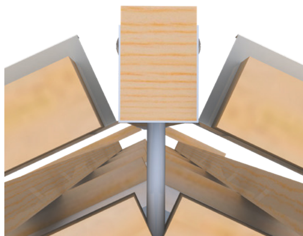
17. Installation of the upper part of the verge trim
