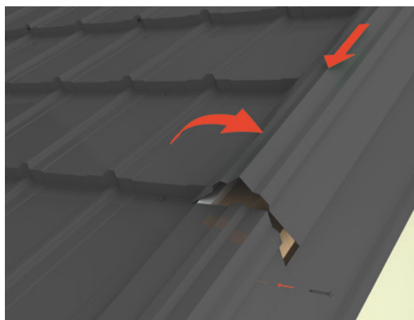
17. Installation of the upper part of the verge trim
