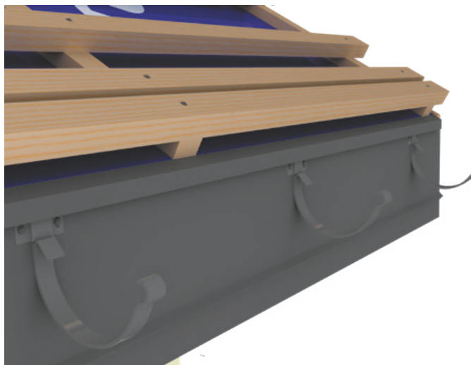
8. Installation of eaves flashing
